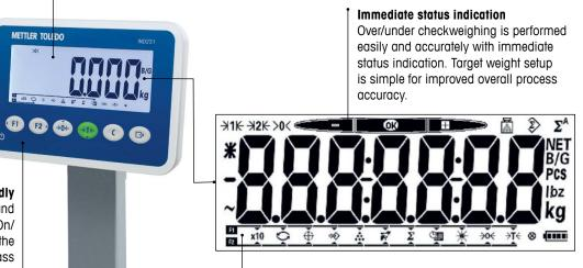
Full control at all times All functions (directly selected over the function keys) and current scale status are always in easy sight providing a good overview for ergonomic operation.
