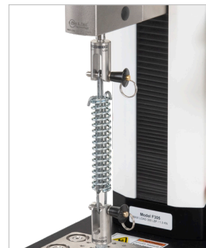
Tension spring testing
